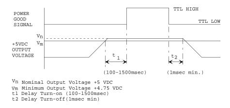
Figure 5-5: Power Good Signal Characteristics
